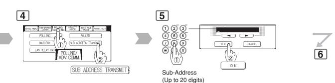
The Sub-Addressing function allows you further routing, forwarding or relaying of document(s) to the desired destinations
